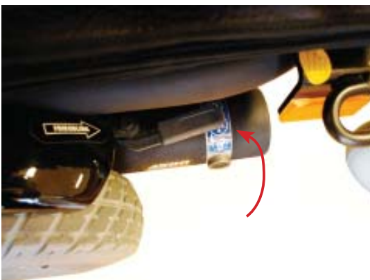
Normal position for driving - pushed in.
