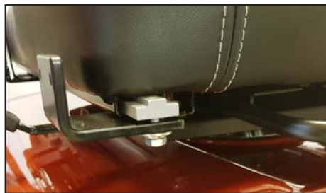
The mounting bracket is slid onto the rail under the seat on the side where the thigh support is to be fitted.
