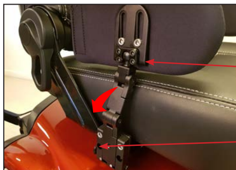
Up/down adjustment is carried out by loosening the two screws in the slots.
