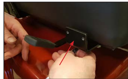
Secure the mounting bracket with two screws.
