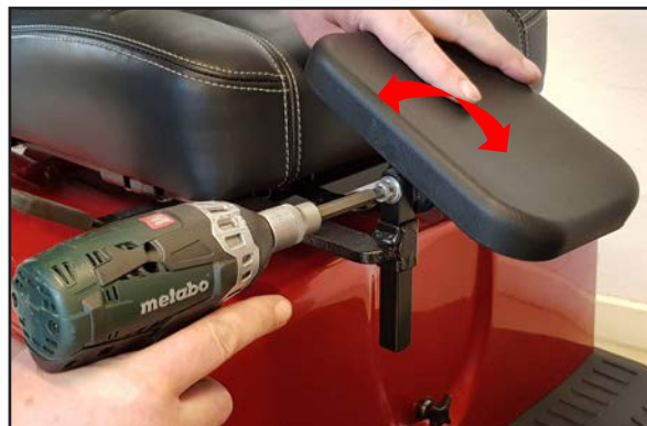
Adjustment of the angle of the amputation support: Loosen this screw – adjust the angle – retighten the screw.
