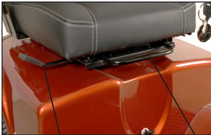
Release lever for seat rotation. Release lever for seat forward/back.
