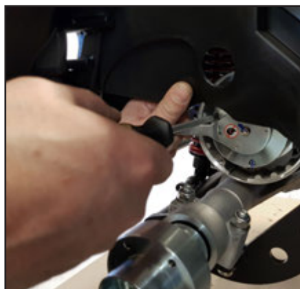
Remove the three screws to dismantle the magnetic brake. They were all greased with locktite when they were mounted.
