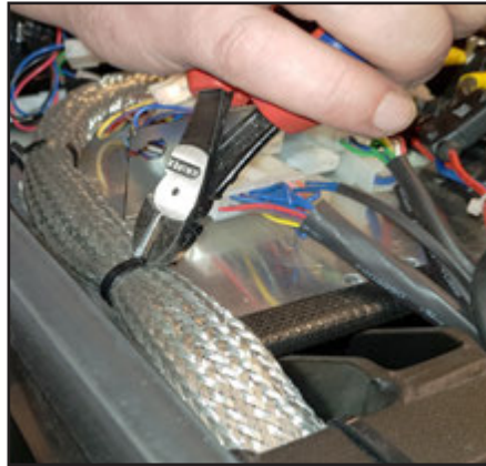
Cut the cable ties that keep the cable in place. Remember new cable ties when mounting again.
