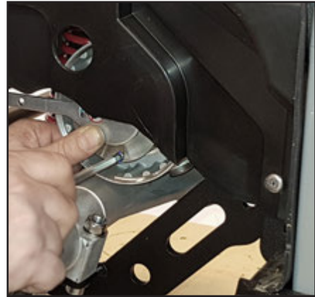
Use locktite on the screws. Tighten the screws with 4 Nm. Locktite No 2400.
