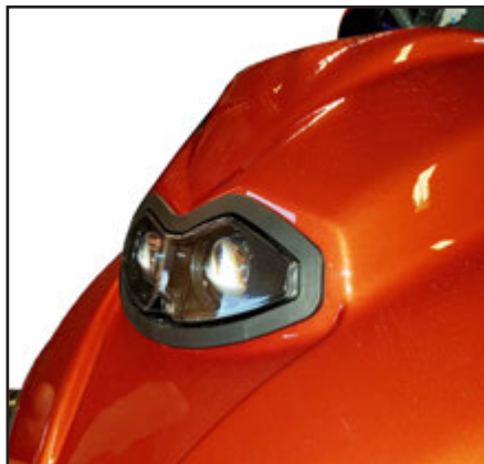
If the headlight stops working, replace the entire headlight.
