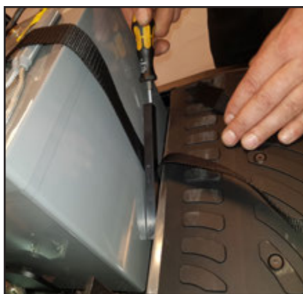
Tilt the spacer, and pull the strap trough.
