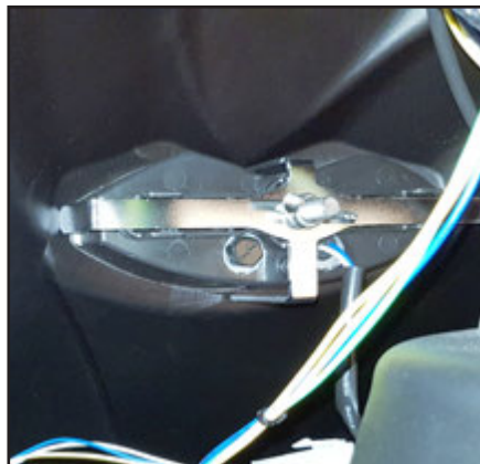
The headlight is attached with a fitting on the back of the screen. A single finger screw holds it firmly in place. Remove the screw.
