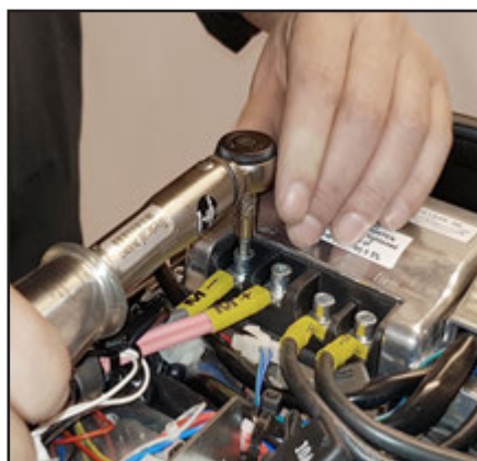
The plugs should be tightened with 5 Nm. Remember to mount new cable ties.
