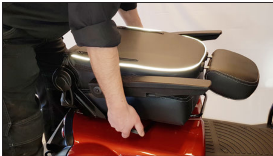
Lift the seat off the seat tube.
