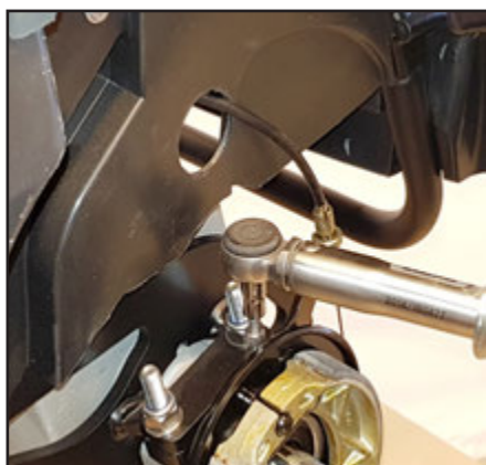
Remount the brake disc. The three screws should be tightened with 4 Nm.
