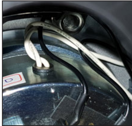
When the new magnetic brake is mounted, be aware to tuck the cable away before mounting the screws.
