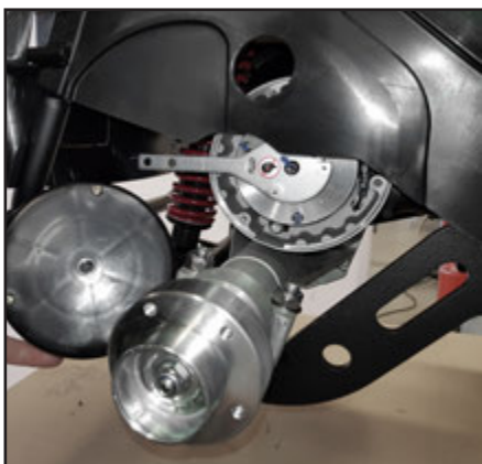
Now there is access to the magnetic brake.
