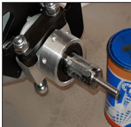
Remove the tape and coat it with bearing grease.
