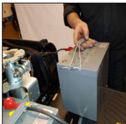
The batteries are now free to be replaced with new ones. Mount in reverse order.
