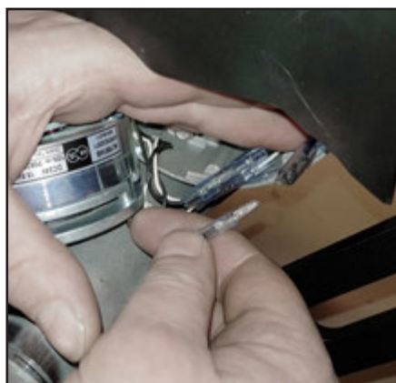
Disconnect the four plugs, and the magnetic is free to be removed.
