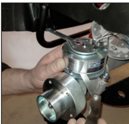
Check the distance to the magnet. If the measure is more than 0,35 mm, it is worn, and has to be replaced. The distance on a new magnetic brake is 0,15 mm.
