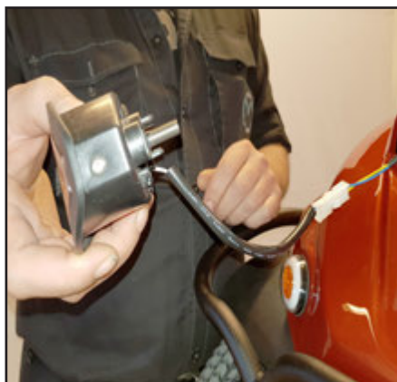
Remove the headlight. Detach the plug, and it is free to change.
