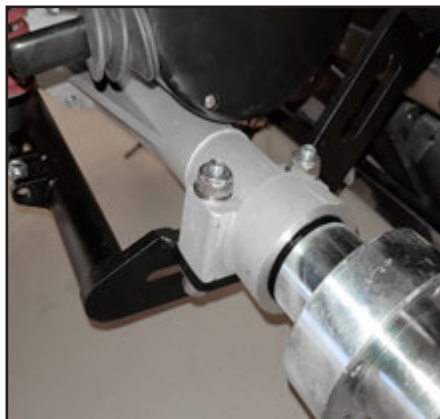
In one side the transaxle is laying on top of the rear suspension. In the other side it is fixed from beneath. Remove the screws from this side first.
