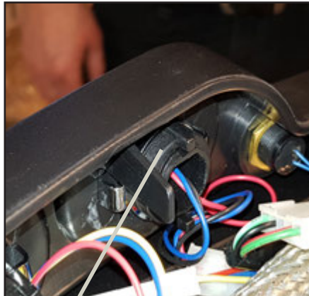
Turn the nut until the tail light is loose.
