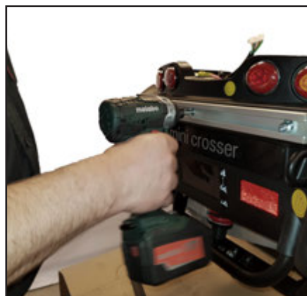
Remove the rear cover. Remove the stopper, and slide of the rubber. Unscrew the three screws. Unplug all electric connectors and the cover is free.
