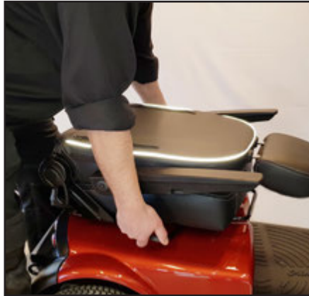
Lift the armrests up, and fold the seat completely. Release the seat turn - turn the seat a little and lift it of.
