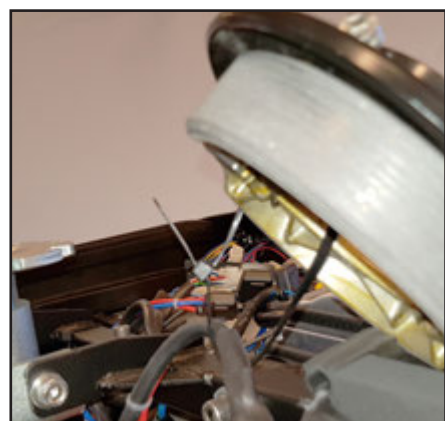
Use a long cable tie, to keep the brake dick away from the working area.
