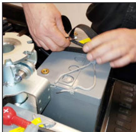
Remove the battery straps.
