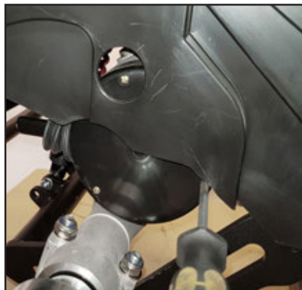
Remove the cover - three screws.
