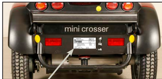
Position of serial number plate on vehicle.
