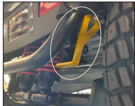
And push up to reactivate the motor (normal driving now possible).
