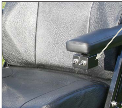
Electric functions by switch box.
