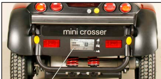
Position of serial number plate on vehicle.
