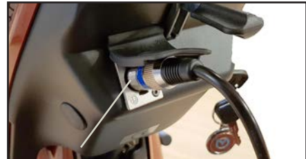
Connect the charging plug to the 3-pin socket on the steering column. The charging socket is located under the protective cover.
