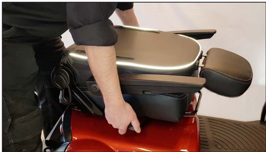
Lift the seat off the seat tube.
