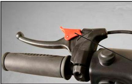
*When using the handbrake as a parking brake, lock it in braking position by pressing the button in while applying the brake. To release the brake, press the button again.*
