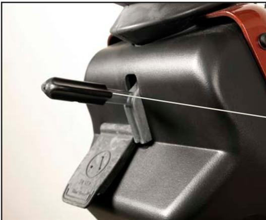
Adjusting the height of the handlebars. Applies to both the 3W and the 4W model.
