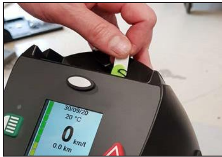
Remove the USB connector..
