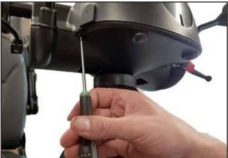
Four screws holds the head. Use tool Torx 10.
