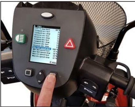
Scrol down in the service menu untill You find P&G menus. Find the "Max fwd speed fast".
