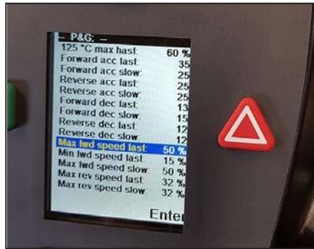
If there is no communication, a lot of theses values will be "1". If that is the Case – go directly to - "Replacing the X2 head". Or: Use "Enter" to change the value. Use the "-" (minus) button untill the value is "50%". Press "Enter" again to accept the new value.
