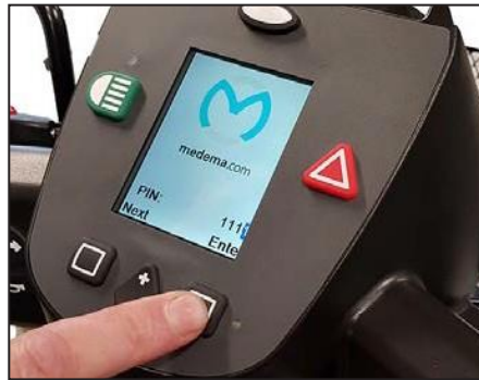
Use the "+" button and "Next" button to enter the code 1111. Finish with "Enter".
