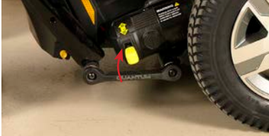
Normal position for driving - pushed up
