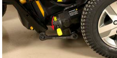
Position for disengagement - pushed down
