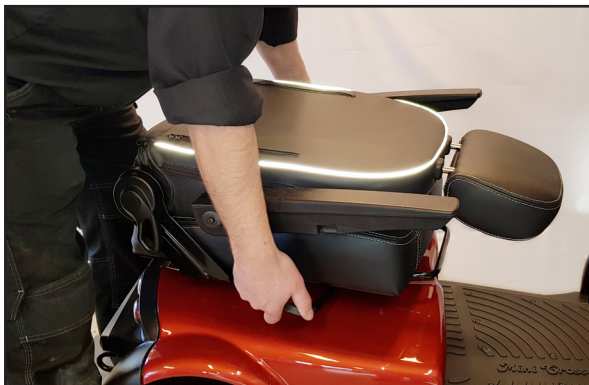
Remove the seat. Release the seat swivel - turn the seat slightly and lift it off. Be careful of your back.
