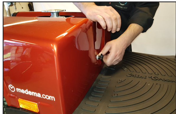
Remove the battery cover. Remove the thumbscrew and pull off the battery cover.
